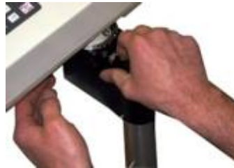
Attach coin catcher tube holder (replace knob to lock into place)
